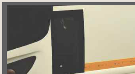
Peep Window for Better Visibility on Sides
