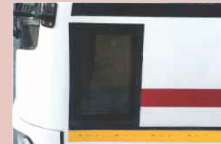
Peep Window for safe driving & better side view
